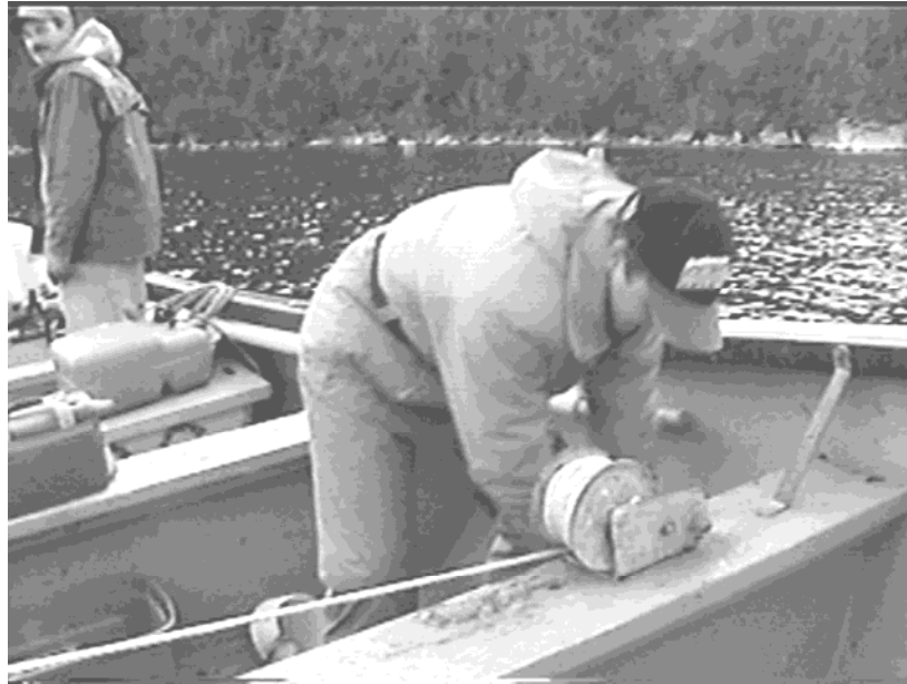
Figure 7.8: Simple hand or trailer winch used to haul mainlines to the surface. This system may be suitable for line maintenance or inspection but is not advised for commercial scale harvests.
